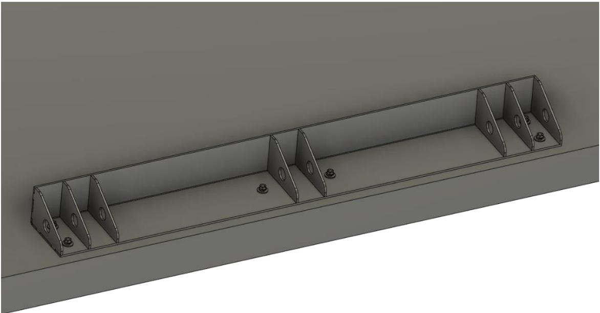
Care must be taken in choosing bolt locations to ensure there are no obstructions under the truck deck that would not allow the hardware to fit properly in place. The underside of the truck deck should be examined, and measurements taken to ensure proper bolt locations are made.
