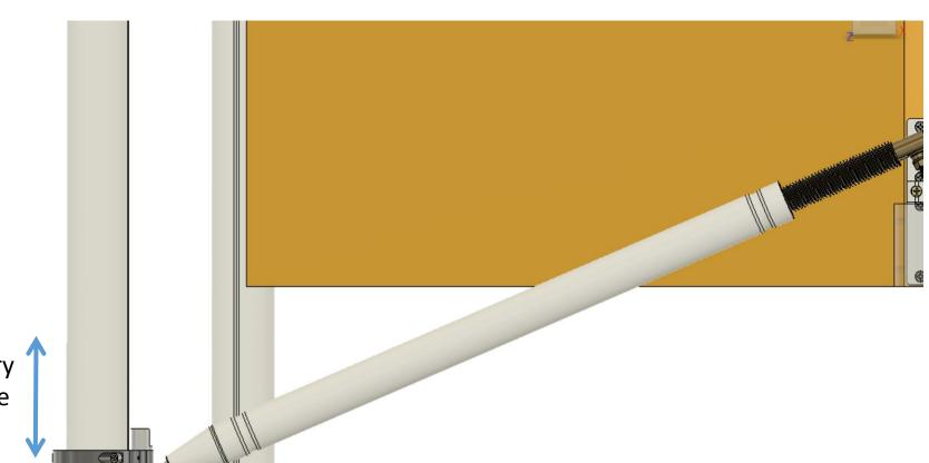
Vertical placement of jack clamp will vary depending on the maximum angle of the front tube.
