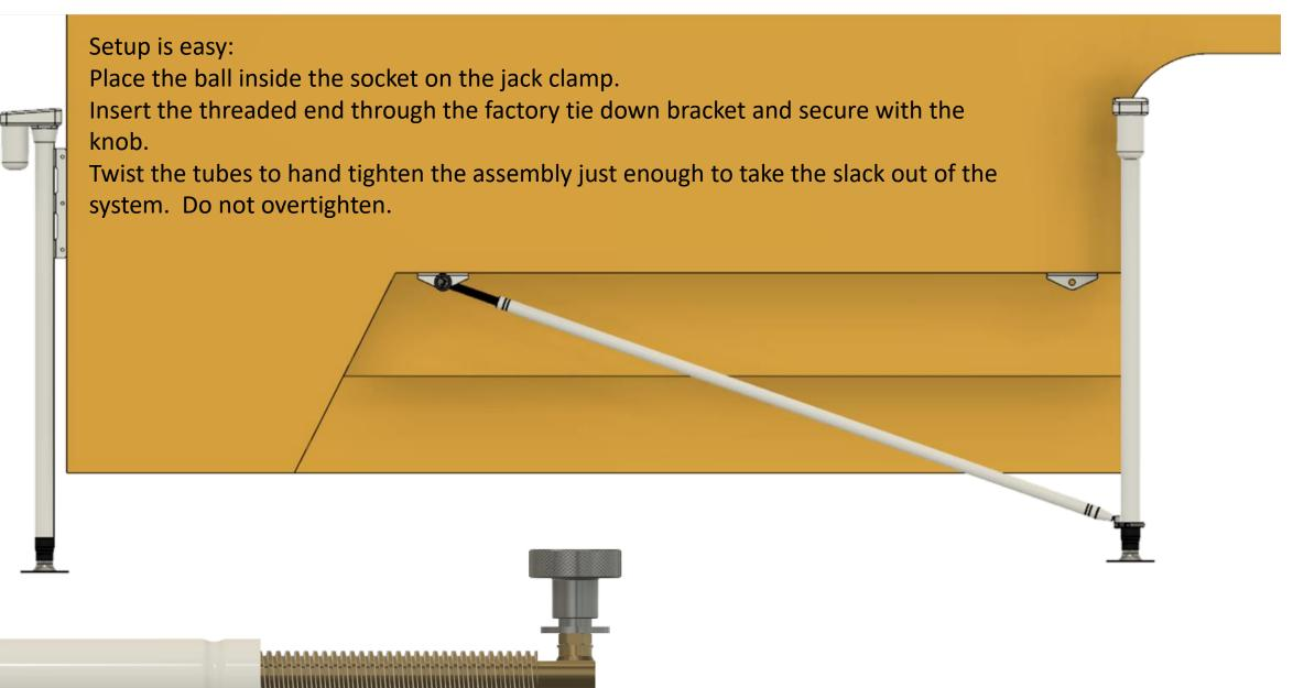
For the front tubes, rotate the tube from the storage position on the front storage hook and place the ball inside the socket on the jack clamp.
