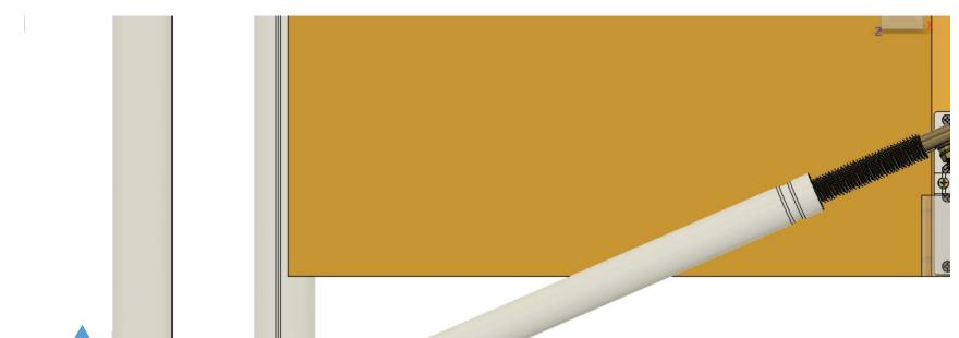
Vertical placement of jack clamp will vary depending on the maximum angle of the front tube.
