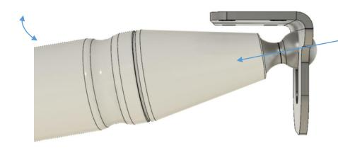
2. The ball now has clearance to be removed or inserted into the mount.
