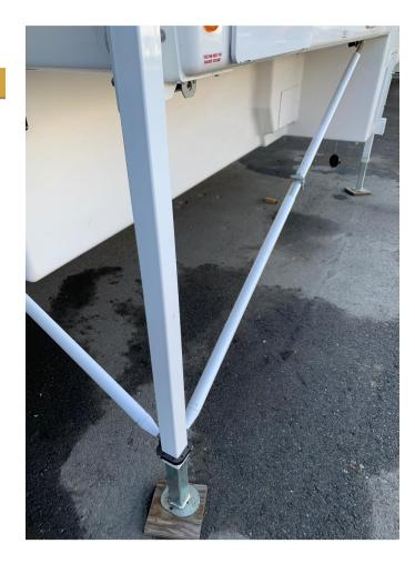
For the front tubes, rotate the tube from the storage position on the front storage hook and place the ball inside the socket on the jack clamp.
