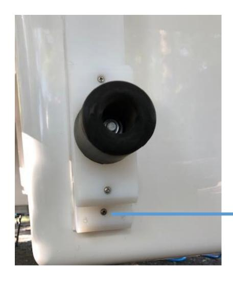
\*\*Please note the Northern Lite set was designed so that there is no drilling into the fiberglass exterior of the camper. The front mounts are secured with the included hardware into the UHM plastic strip as shown on the following page.
