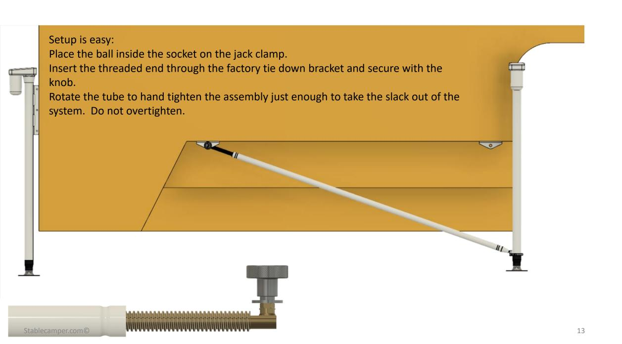
For the front tubes, rotate the tube from the storage position on the front storage hook and place the ball inside the socket on the jack clamp.
