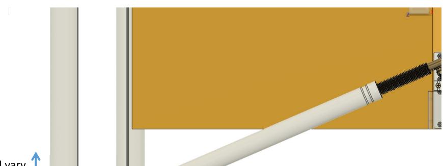
Vertical placement of jack clamp will vary depending on the maximum angle of the front tube.
