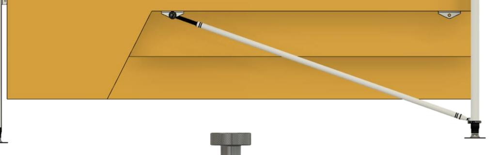
For the front tubes, rotate the tube from the storage position on the front storage hook and place the ball inside the socket on the jack clamp. Twist the tube to tighten the assembly.
