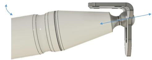
2. The ball now has clearance to be removed or inserted into the mount.
